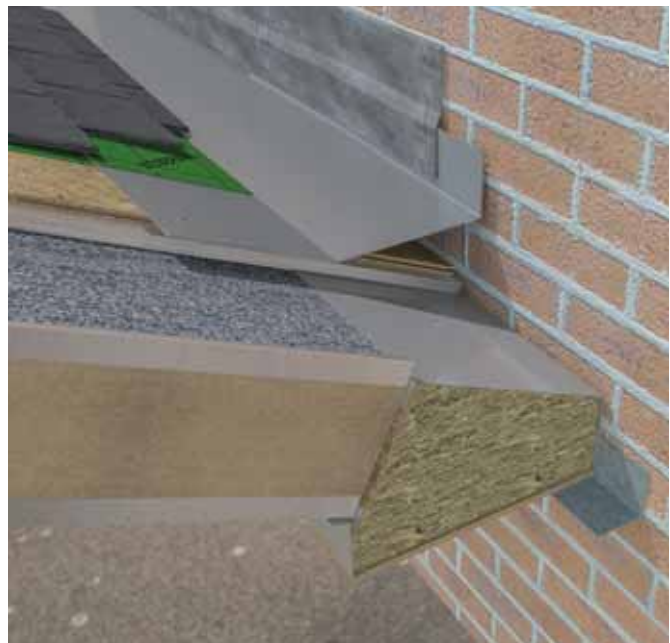
Tapered box gutter
